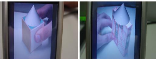
**Figure 5:** Handheld augmented reality results using the developed markerless 3D tracker.
